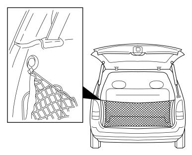
The cargo net helps stabilize lightweight objects in the cargo area. Attach the net to the anchors provided. The cargo restrained in the net must not exceed 22 kg (50 lbs.) or the net may not stay secured.
